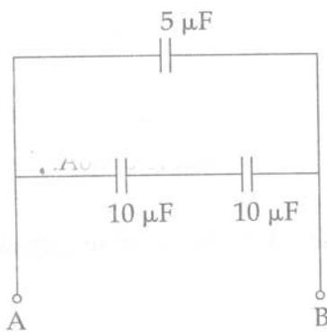
Calculate the effective capacitance of the capacitors shown in figure.
